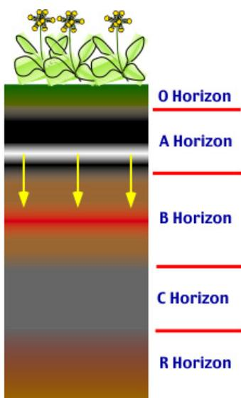
Figure 1: A typical soil profile
