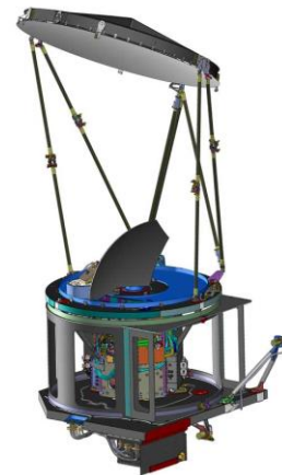
Figure 4: GPM Microwave Imager (GMI) is a passive radiometer with an antenna above.
