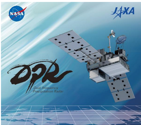
Figure 3: The Dual-Frequency Precipitation Radar (DPR) is the two boxes on the bottom of the Core Observatory – the small one is the Ka frequency radar and the larger flat box is the Ku frequency radar
