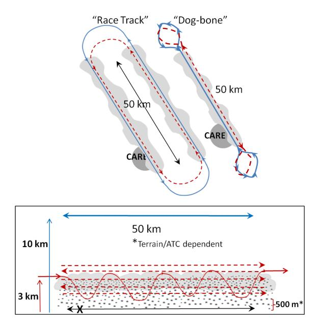
Figure 12: Sample coordinated aircraft observations for Lake Effect Snow sampling. Citation (red dash)porpoise or stair step in altitude over 50 km leg from 1.5 kft – 10 kft (~500 m to 3000 m). DC-8 (blue solid lines) constant altitude oval orbit over Citation (DC-8, 50 – 75 km leg; altitude 33 kft (10 km) nominal). Legs stretch to the north-northeast with CARE site at southern end (hit other sites as possible). Note that porpoising pattern is not to scale (exaggerated to illustrate concept).
