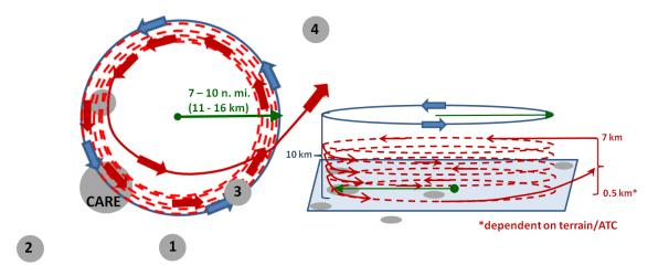
Figure 13: Sample coordinated aircraft observations for Synoptic Snow sampling. Citation (red dashed lines)-Spiral descent from TBD altitude 7 km (24 kft nominal) to 0.5 km (1.5 kft). DC-8 (blue lines) fixed circular orbit over Citation (DC-8 altitude 33 kft nominal)
