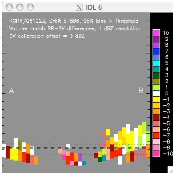
Figure 11. As in Fig. 10, but with a +3 dBZ calibration correction to the GV reflectivity.
