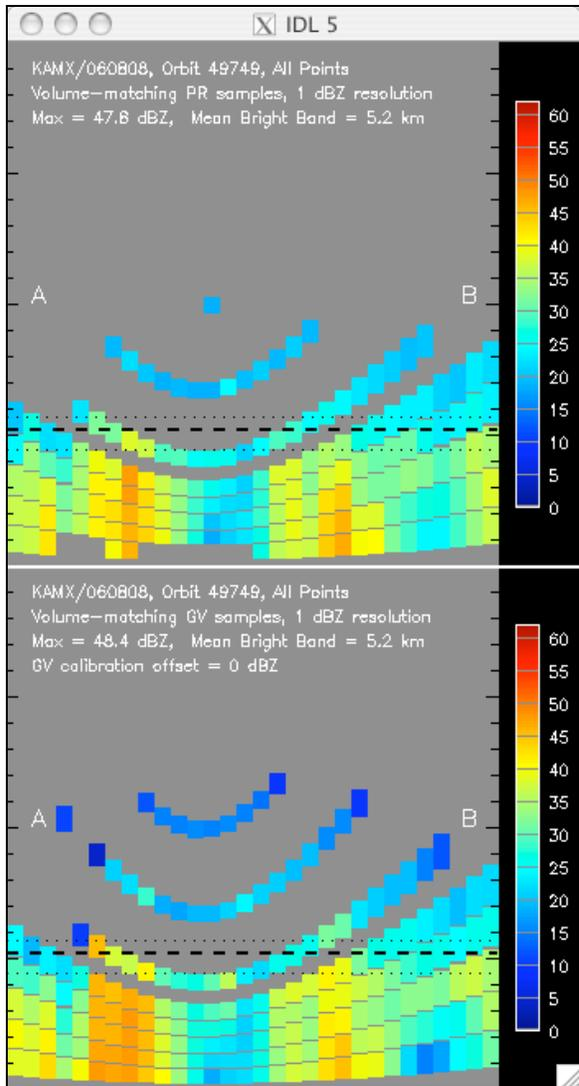
**Figure 4. Vertical cross sections of geometry-matched PR (top) and GV (bottom) data along PR scan line through the user-selected location. All available samples are shown in this example (i.e., PCT\_ABV\_THRESH=0).**
