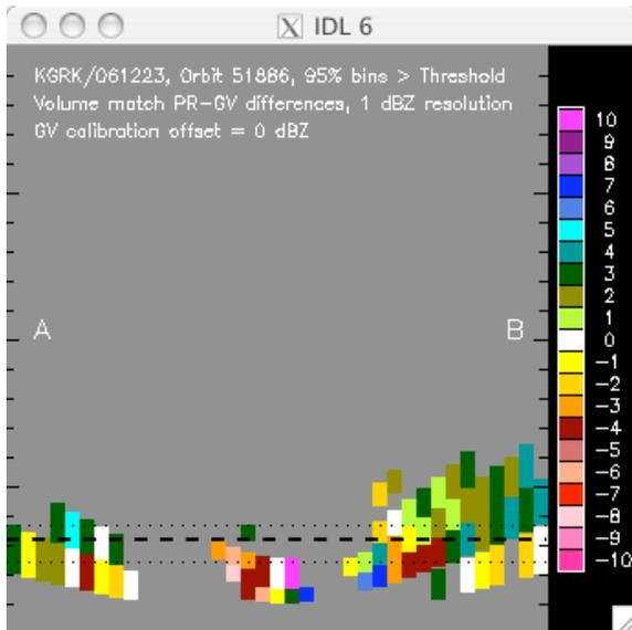
Figure 10. PR-GV difference cross section for the KGRK WSR-88D radar with 0 dBZ GV offset.
