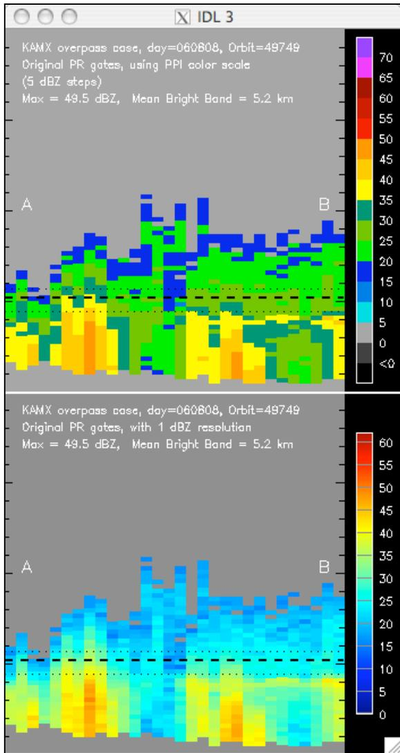
**Figure 6. Vertical cross section of full-vertical-resolution (250 m) PR reflectivity data from the original, unaveraged 2A-25 attenuation-corrected reflectivity, for the case shown in Figs. 3-5. The same data are plotted in both panels – only the color table is different between the two.**
