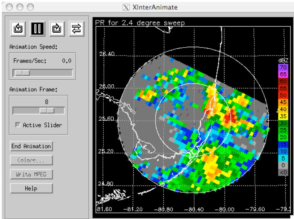
**Figure 7. One PR frame of a PR and GV animation loop, showing volume-matched PR data for the 2.4 degree elevation sweep of the GV radar.**
