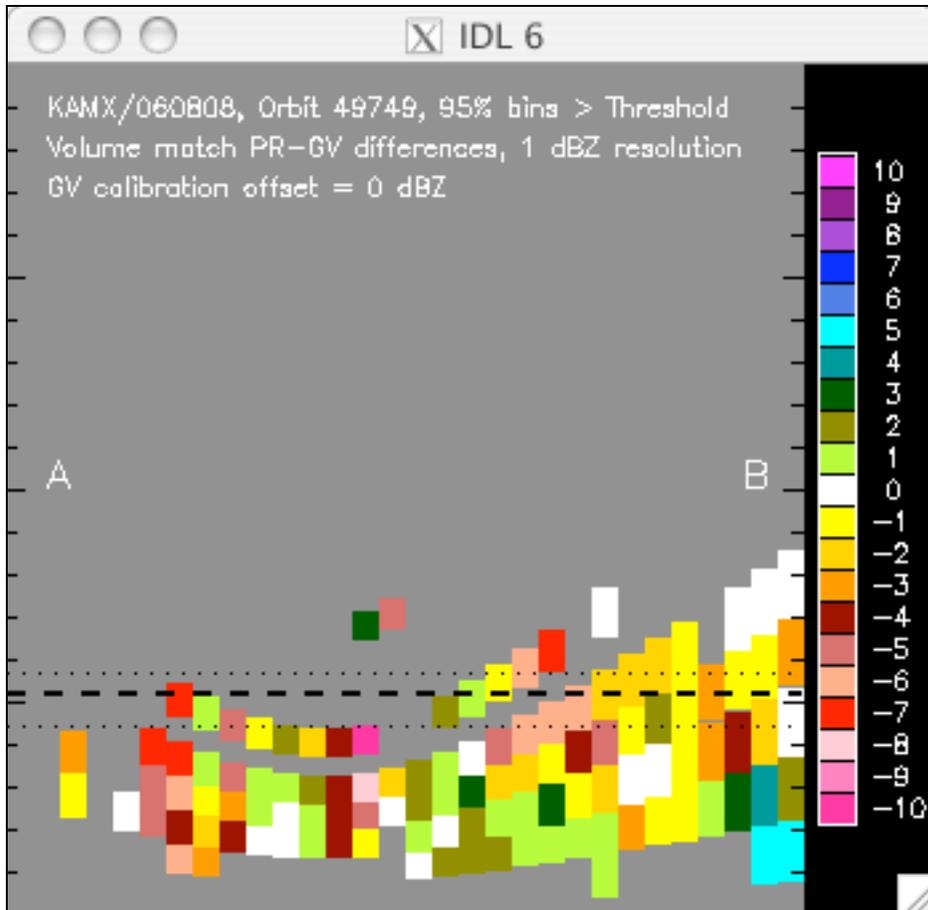
**Figure 14.** As in Fig. 5, but limited to those samples where at least 95% of the PR and GV bins in the volume averages meet the reflectivity thresholds.
