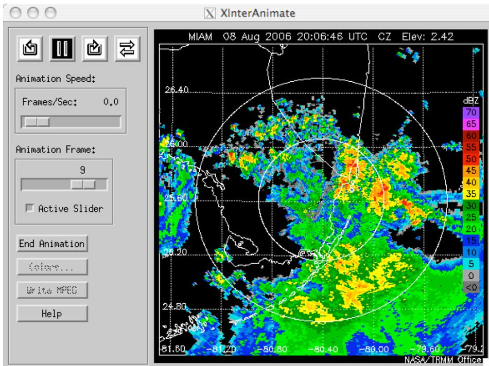
**Figure 9.** Full-resolution GV PPI from the original UF radar data file, if available, is interleaved with corresponding PPIs of volume-matched data (Figs. 7, 8) in the animation loop.
