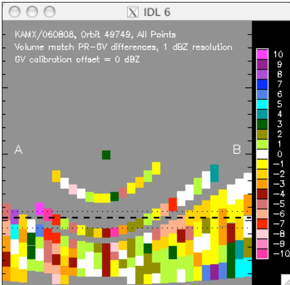
Figure 5. Cross section of reflectivity difference, PR-GV, from volume-matched data, for the case shown in Fig. 4.
