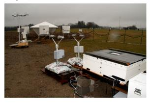
**Fig 1:** CARE site near Egbert, Ontario. Shown in the foreground are the low profile 2D video disdrometer and the two Parsivels. The POSS is in the background to the left of the view which is from the SE.
