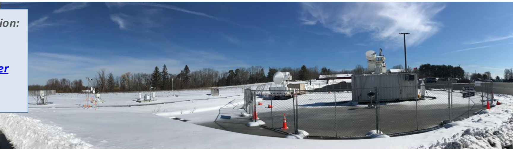
UCONN Field site: GPM GV instruments include K-band and W-band profiling radars and Ka-Ku band scanning radars, weighing and tipping bucket pluviometers, laser disdrometers, and high-speed and high-resolution cameras. Credit: D. Cerrai
