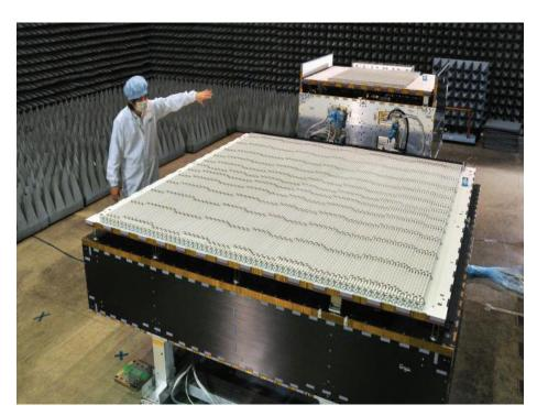
A JAXA scientist standing next to the Dual-frequency Precipitation Radar (DPR) instrument. The Ku-band radar is in the foreground and the Ka-band radar is the smaller one in the background."
