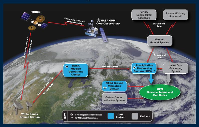
The GPM mission ground system includes all the assets needed to command and operate the GPM Core Observatory in orbit, as well as manage and distribute data received from the Core and other satellites in the constellation.
