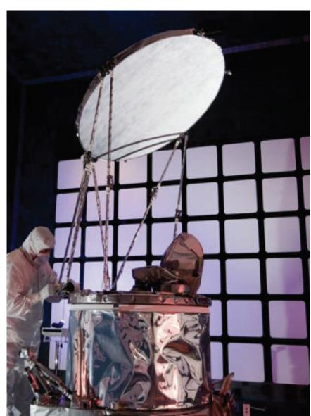
GMI undergoes electromagnetic interference and compatibility testing at Ball Aerospace & Technologies Corp.
