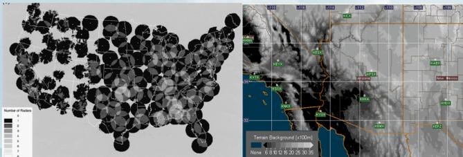
Figure 1. (left) Effective WSR-88D radar coverage at a constant height at 3km Above Ground Level [from Maddox et al. (2002)]; (right) DEM of the state of Arizona. It also shows the sparse distribution of ground radars.
