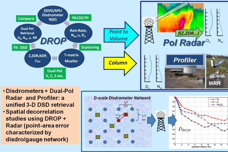
Disdrometers + Dual-Pol Radar and Profiler: a unified 3-D DSD retrieval
