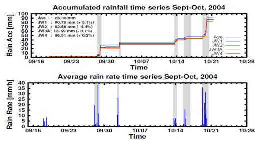
The rain accumulations of the individual disdrometers show noticeable differences from the areal mean with a maximum percent absolute bias of 12.6% for JW2 (S02).
