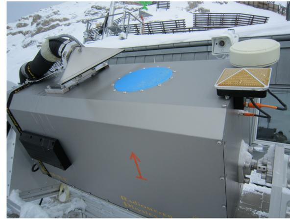
**Dual Polarization Radiometer (DPR)
