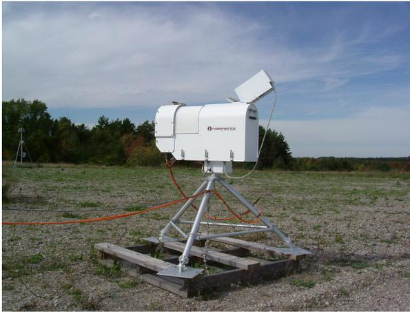
**TP3000 profiling radiometer
