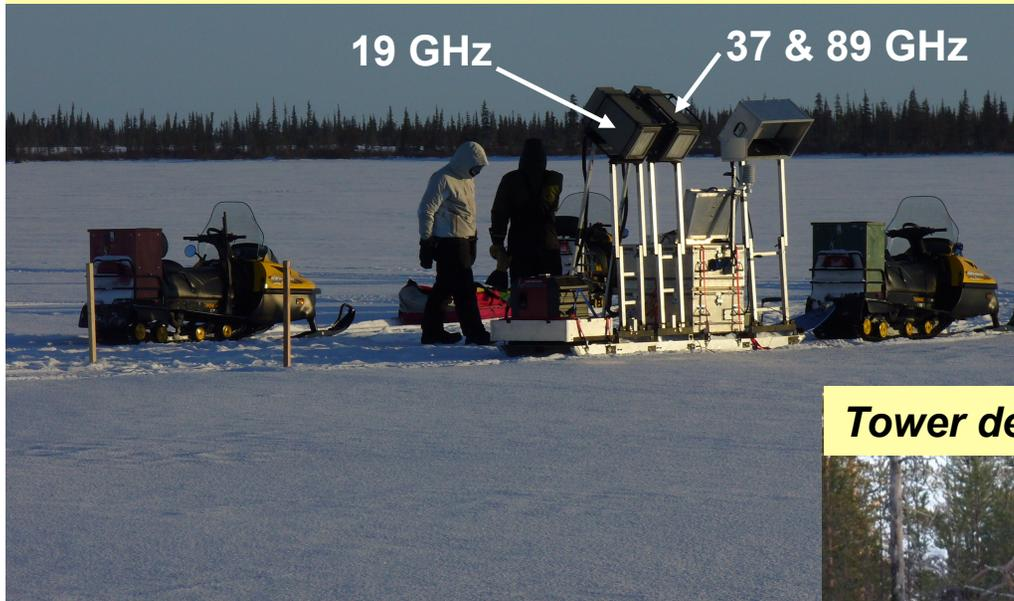
19, 37, and 89 GHz (dual-pol) radiometers will be deployed on a tower for continuous measurements of the surface during the snow cover season.
