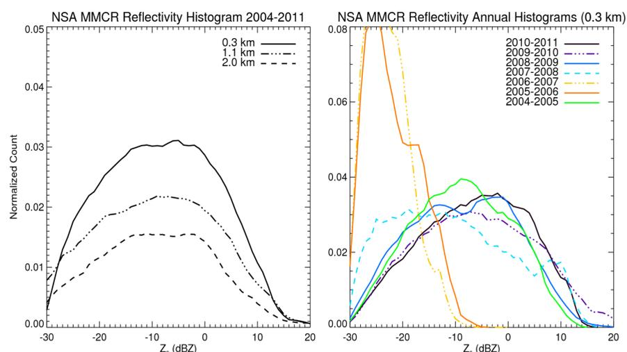
**Fig. 3:** Radar reflectivity histograms for the 2004-2011 dataset shown at various heights AGL (left) and annual histograms at 0.3 km AGL (right).
