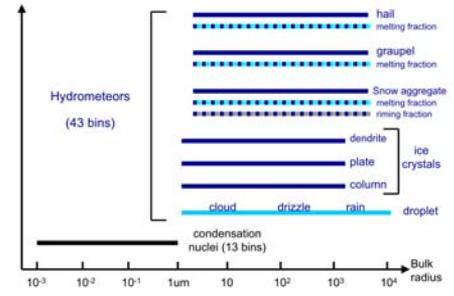
We implemented spectral bin microphysics (SBM) for cloud based on the Hebrew University Cloud Model (HUCM) (Khain et al., 2011) into the Weather Research and Forecasting model (WRF) ver. 3.4. The SBM explicitly prognosticates mass liquid fraction of each bin of melting snow aggregates, graupel and hail (Phillips et al., 2007). The WRF-SBM was employed in 36-hours real-time simulations using online 2-way grid nesting configuration for the domains 2 and 3.
