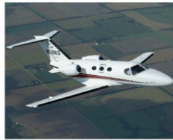
5-person corporate jet (Citation Mustang) Wingspan 43' Takeoff weight (max) 8635 lbs
